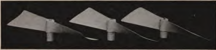
Fig. 11.—The three best screws. The screw on the right has a uniform pitch throughout, the middle screw has increasing pitch, and the left screw compound increasing pitch.
